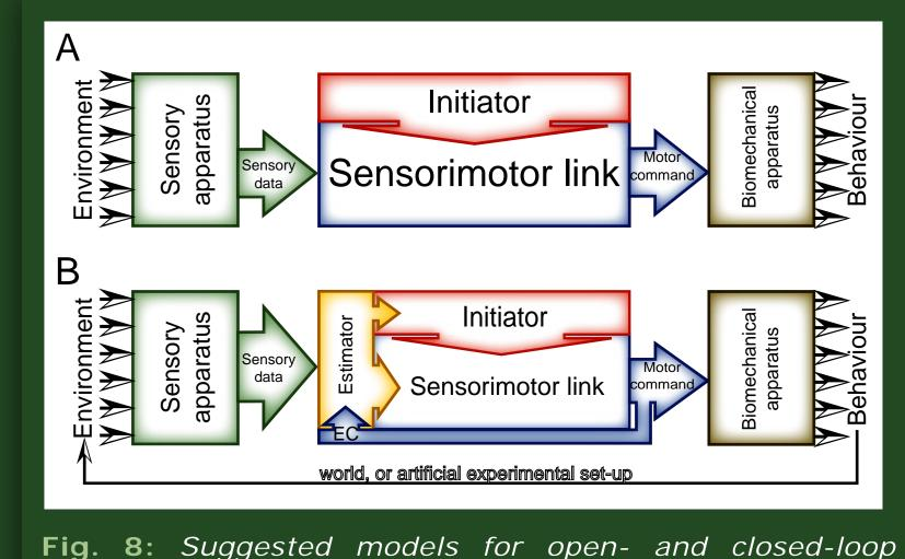
experiments. A - Open-loop model as proposed in Fig. 1 (for the *openloop* group). B - Closed-loop model (for the onestripe and uniform groups). Performance in a situation with a closed reafferent feedback loop is commonly modelled with a state estimator (often approximated by a Bayesian Kalman filter), cross-correlating sensory input with recent motor commands via an efference copy (EC). Such an evaluation is required for efficient behavioral control of incoming sensory data.
