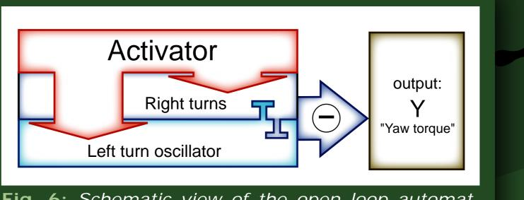
Fig. 6: Schematic view of the open loop automat. The activator sends excitatory input to both turn generators. The turn oscillators inhibit each other. The output is the difference signal between the left and right turn oscillator. Each oscillator is described by a logistic map, and the coupling modulates the individual parameters of each map.
