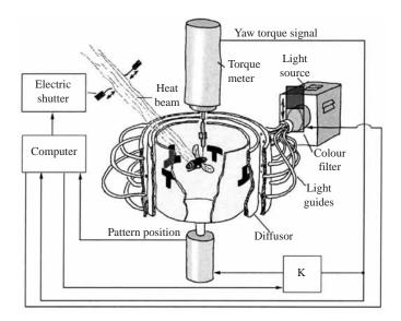
Fig. 1. The flight simulator. The fly is flying tethered in a cylindrical arena homogeneously illuminated from behind. The fly's tendency to perform left or right turns (yaw torque) during tethered flight is measured continuously and fed into a computer. The computer controls background pattern position, heat beam shutter closure and the colour of illumination according to the conditioning rules. K indicates the motor control unit.
